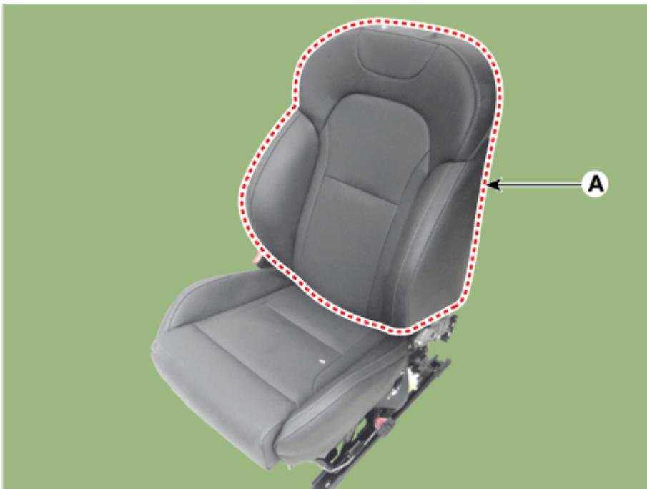
14. Remove the front seat back covering (C) from the front the seat back frame after removing the velcro tape (A) and hog-ring clips (B).
