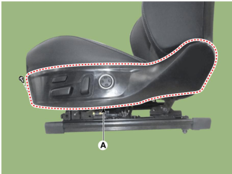
4. Disconnect the front seat power switch connector (A).
